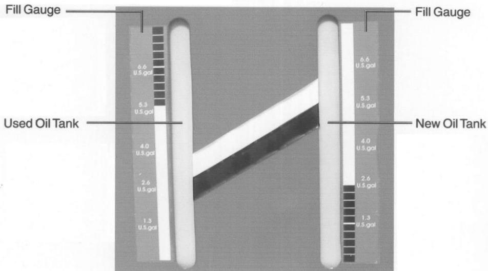
As the tanks are filled, the fluids can be viewed through the tank and measured.
