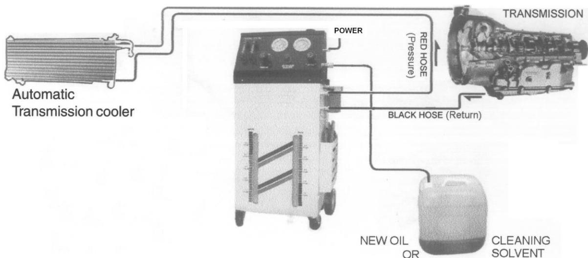
6. Turn the (right) Filling-Recycle Reverse Control knob to the Filling position.
