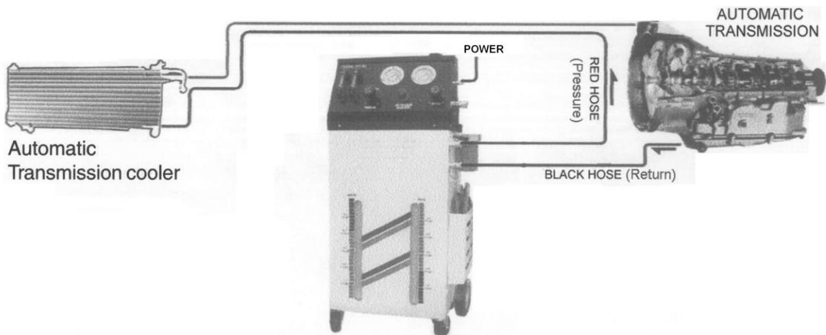
7. During this process, View the new and used oil flow rate. They should flow at equal rates. If used oil flow fast than new oil, please adjust the ball valve fixed on the oil black return line to make them have the same flow rate.
